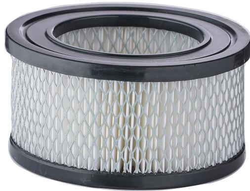
These filters are made with a vinyl material known as "plastisol", which bonds the pleated paper media preventing bypass. They also have soft rubber gaskets to seal the filter in its housing.
