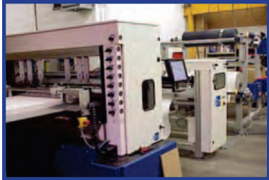
Filtration Systems' Computer Controlled Pleaters make consistent high-quality products.
