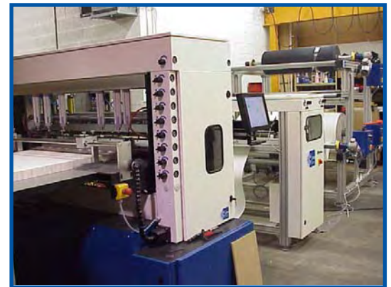
Our Computer-Controlled Pleater makes uniform sharp straight pleats
